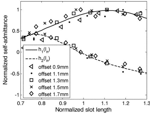
Fig. 5. Normalized self-admittance vs. normalized slot length for the dielectric-covered single-slot sets.
