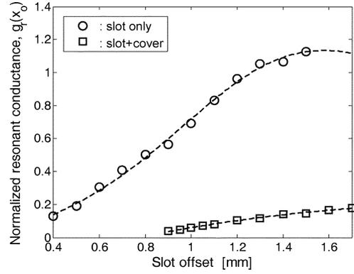
Fig. 3. Normalized resonant conductance versus slot offset for the single-slot sets.
