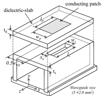
Fig. 1. Geometry of a single-slot set consisting of a radiating slot and a cover structure.
