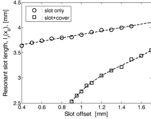
Fig. 2. Resonant slot lengths versus slot offset for the single-slot sets.
