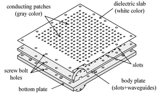
Fig. 6. Geometry of the  $16 \times 16$  slot-array antenna with the cover structure.
