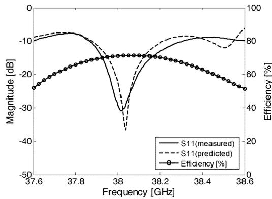
Fig. 7. (left-side) Measured  $|S_{11}|$  and (right-side) radiation efficiency of the  $16 \times 16$  slot-array antenna with the cover structure.
