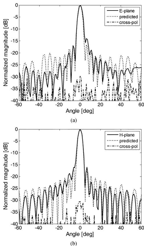
Fig. 8. Measured radiation patterns of the  $16 \times 16$  slot-array antenna with the cover structure: (a) principal E-plane and (b) principal H-plane.
