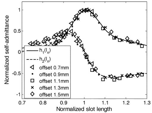
Fig. 4. Normalized self-admittance versus normalized slot length for the uncovered single-slot sets.
