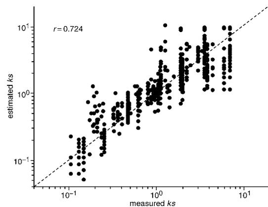
**Fig. 1** Comparison between surface parameter  $ks$  ( $k=2\pi f/c$ ,  $s$ =rms height) estimated by inversion technique and that measured *in situ*
