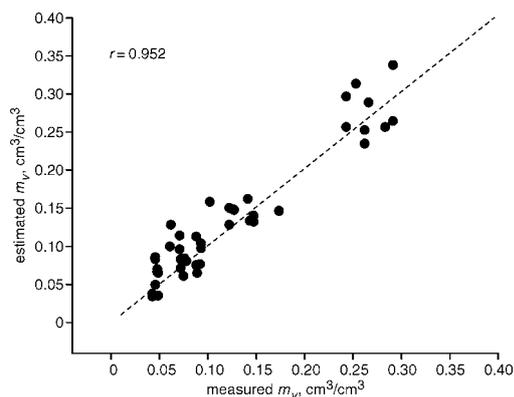
Fig. 2 Comparison between estimated and field-measured volumetric moisture content  $m_v$  for multi-frequency and multi-angle data
