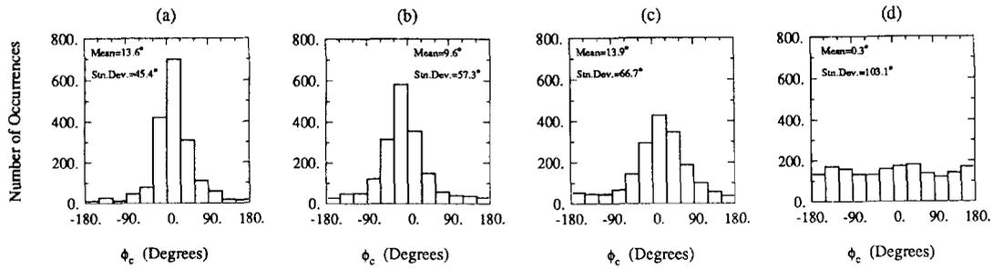
Figure 1: Distribution of co-polarized phase angle  $\phi_{hh} - \phi_{vv} = \phi_c$ , (a) at 1.5 GHz, (b) at 4.75 GHz, (c) at 9.5 GHz, and (d) cross-polarized phase angle  $\phi_{vh} - \phi_{uv} = \phi_x$  at 1.5 GHz, for surface 1 ( $s = 0.4cm$ ) at  $30^\circ$ .
