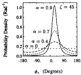
Figure 2: The probability density function of the co-polarized phase angle  $\phi_c = \phi_{hh} - \phi_{vv}$  for a fixed value of  $\zeta$  and four values of  $\alpha$ .
