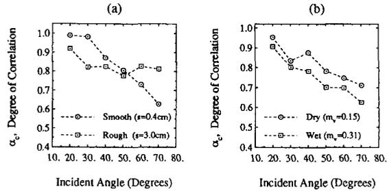
Figure 3: The degree of correlation  $\alpha$  of soil surfaces at 4.75 GHz, (a) for two different surface roughnesses ( $m_v \approx 0.15$ ) and (b) for two different moisture conditions ( $s = 0.4cm$ ).
