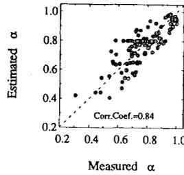
Figure 6: Comparison between the values of  $\alpha$  estimated by the proposed model and those measured using scatterometers for the data set used in development of the model.
