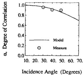
Figure 5: Empirical model compared with an independent data set measured at 5.3 GHz for a surface with  $s = 0.78cm$  and  $m_v = 0.07$ .
