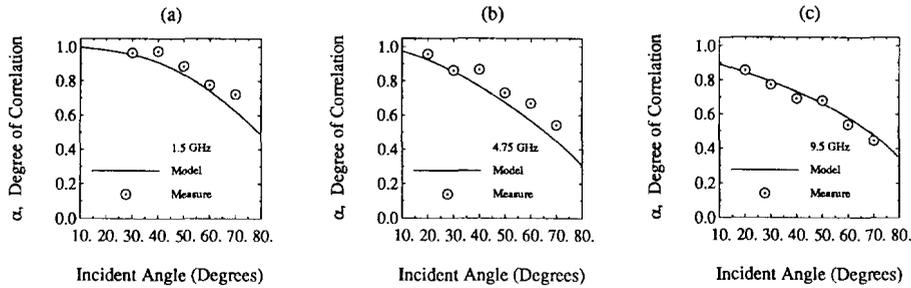
Figure 4: Empirical model compared with the measured data for surface 1 ( $s = 0.4cm$ ) with  $m_v = 0.29$  at (a) 1.5 GHz, (b) 4.75 GHz, and (c) 9.5 GHz.
