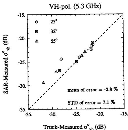
Fig. 11. Comparison of POLARSCAT with AIRSAR corrected data. The JPL AIRSAR data have been calibrated using the POLARSCAT data for the very rough field. The data for the remaining fields are plotted at *L* band.
