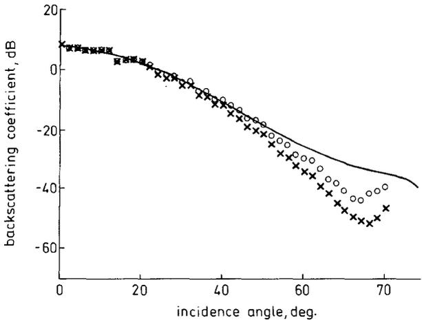
**Fig. 6** Backscattering coefficients computed by tapered illumination method and new formulation of Kirchhoff approximation
