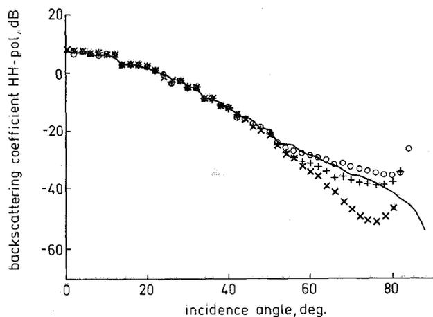
**Fig. 8** Backscattering coefficients ( $\alpha_{hh}^0$ ) computed by new numerical technique and tapered illumination technique
