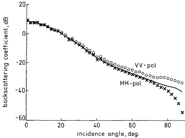
**Fig. 5** Comparison of backscattering coefficients as computed by new numerical method and new formulation of Kirchhoff approximation
