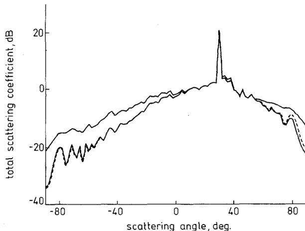
**Fig. 3** Total bistatic scattering coefficient (coherent + incoherent) for surface with  $ks = 0.3$  and  $kl = 3.0$ . Both polarisations are shown for incidence angle  $\theta_i = 30^\circ$  and the effect of the width of tapered resistive sheet is also examined. Resistive sheet length: —  $1\lambda$ , VV-pol; - - -  $3\lambda$ , HH-pol
