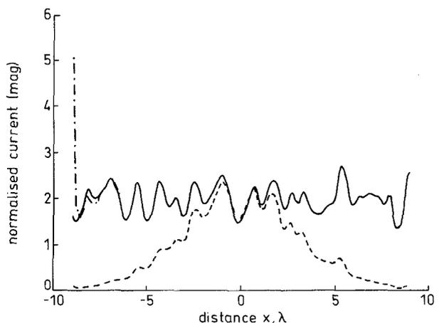
**Fig. 7** Comparison of normalised current distributions computed by new numerical technique and tapered illumination technique
