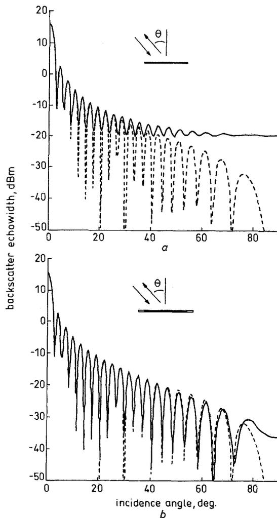
**Fig. 2** Backscattered echowidth of flat conducting strip (width =  $10\lambda$ )
