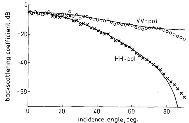
**Fig. 4** Comparison of backscattering coefficients as computed by new numerical technique and first-order small-perturbation solution. For a surface with  $ks = 0.15$  and  $kl = 2.0$  ( $N = 40$ ,  $D = 14\lambda$ ,  $\Delta x = 0.1\lambda$ )
