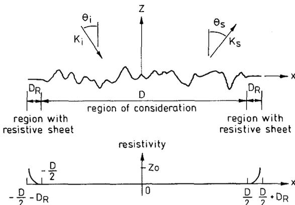
**Fig. 1** Sample surface loaded with resistive sheets, and resistivity function profile
