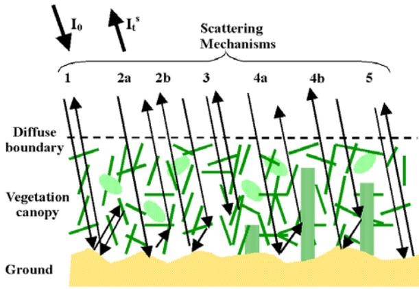
Fig. 1. Scattering mechanisms.
