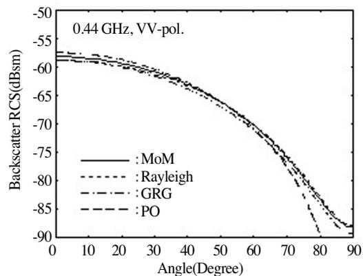
Fig. 3. Comparisons of analytical and numerical backscatter cross sections of a leaf at 0.44 GHz and VV-polarization.
